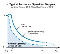
Steppers: Stepper motor drive systems are used very successfully in many office and industrial automation applications. Properly applied they are typically the most cost-effective solution to a Smart Motion application. If their characteristics are misunderstood and they are mis-applied, costly applications failures frequently result.
