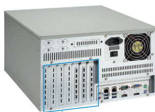
Flexible I/O opening ▲ Rear view
